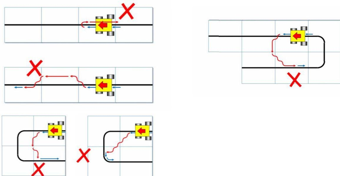
Fig.9. Examples of lost line by the robot.
